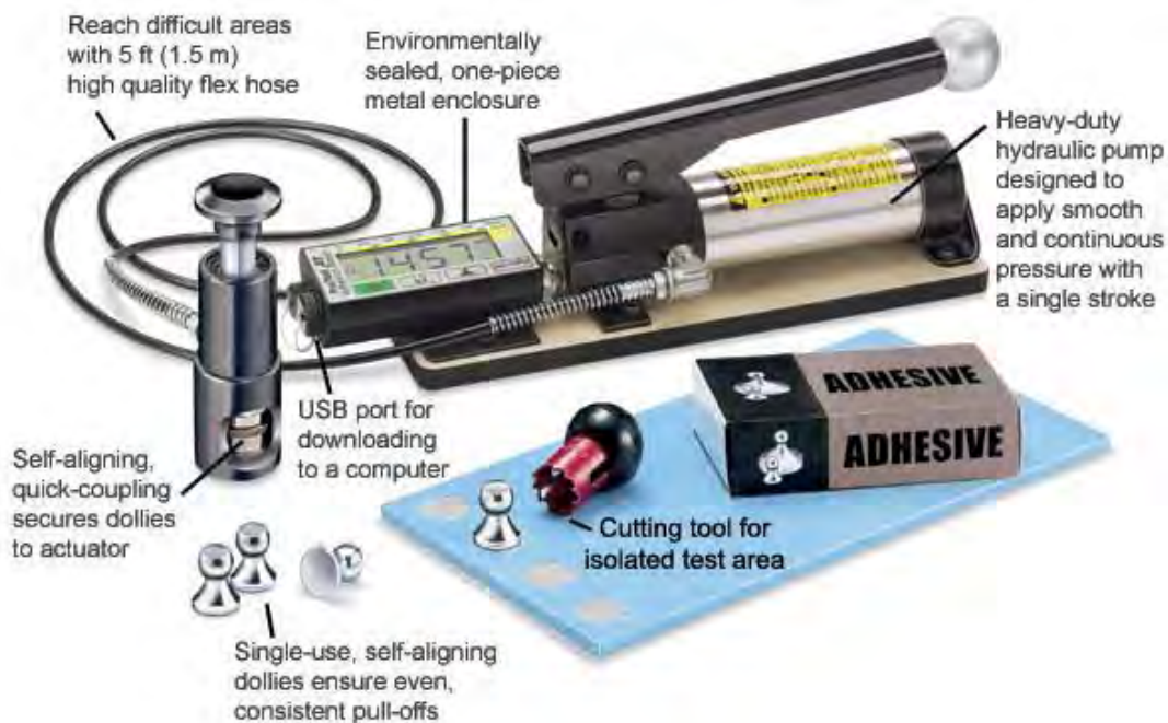
Figure 1. The PosiTest AT Measures adhesion of coatings to metal, wood, concrete and other substrates featuring a manual hydraulic pump designed to apply smooth and continuous pressure with a single stroke [1].
